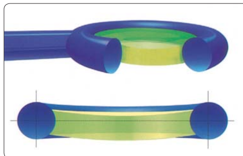
Depth or thickness of the loop wall, and the internal diameter, are critical parameters that control the actual volume delivered by the loop (i.e., internal diameter + wall depth [thickness] + surface tension = actual volume carried).
