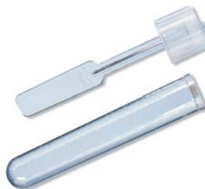
Falcon™ SWUBE™ Pinworm Paddle features a removable paddle designed for direct examination via microscope.
